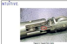
Figure 6: Frayed Pitch Cable
