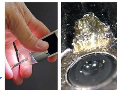
Figure 5: Enhanced magnification microscope and identified damage (exposed glass light fibers)
