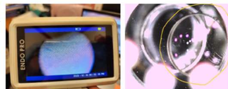
Figure 4: Endoscopic video verification tool with identified damage (dislodged lens within the rigid endoscope)
