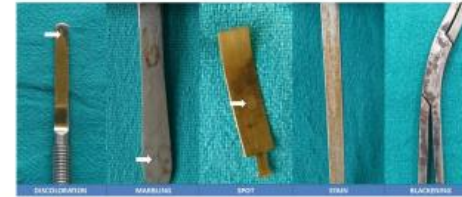
Figure 1. Images showing patterns of common changes seen within the instruments.
