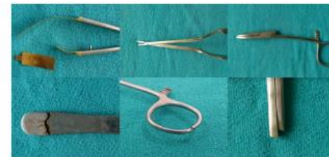
Figure 4. Images showing different sites of fractures sustained within the instruments.
