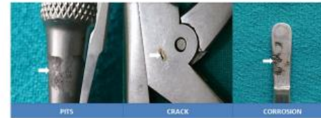
Figure 2. Images showing pits, cracks and corrosion affecting the instruments.
