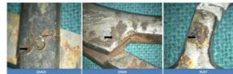
Figure 3. Images showing damages sustained within the instruments under magnification.
