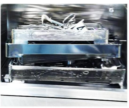
Should you fill the chamber up to the top with instruments?
